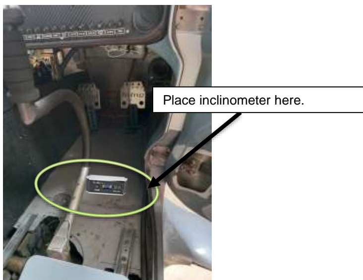
Figure 3: Transverse levelling reference position.
