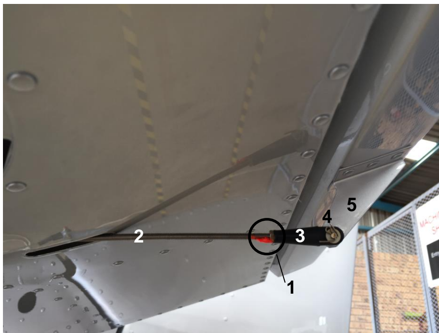
Figure 31: Elevator control horn (5)
